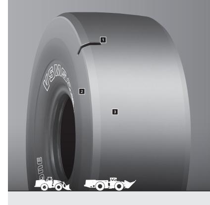
The Steel Smooth Tread Mine Service 2 radial tire is ideal for severe operating environments requiring maximum cut resistance and long tread wear contributing to lower operating costs.
